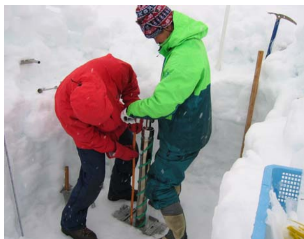
Photo 2 Drilling an ice core using a hand auger.
