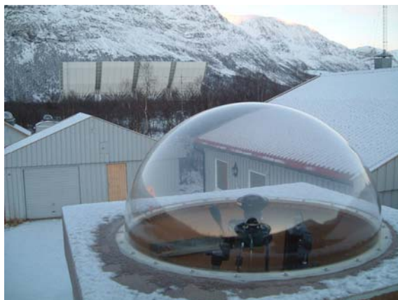
Fig. 4 The all sky camera installed in Tromsø.
